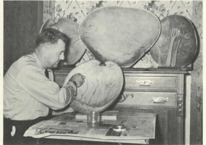
ALMOST DONE WITH THIS ONE . . . Final step in finishing burl is to apply coating of oil to inside, turpentine and varnish to outside of bowl. Three finished bowls on sideboard, center one measures 30" across.
