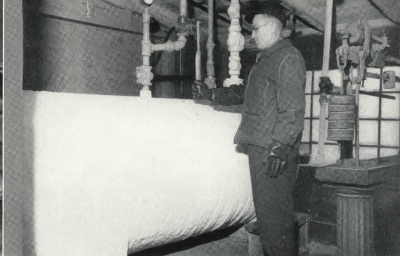
11. Chlorine is weighed in this frost-covered tank before shipping in containers. Shown here is Peter Cantin.
