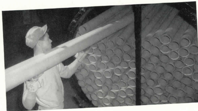
6. Roy Byrd loads tubes into huge tank for pitch treating under vacuum.
