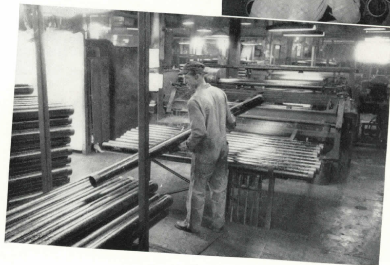
11. George Page, truck operator, is shown hauling treated tubes to finishing lathe.
