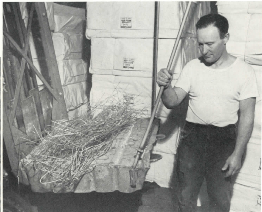
Ayotte is shown here removing poles from rack so that wire may be brushed off without being lifted.
