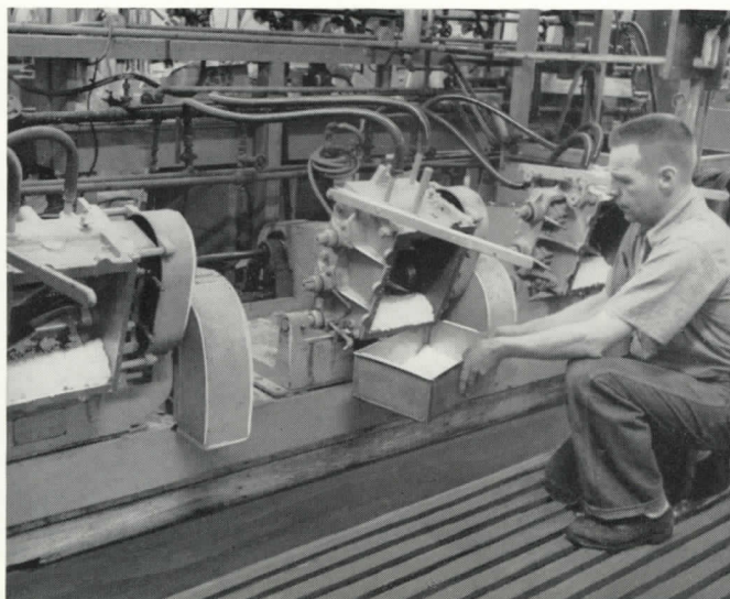
Jerry Vallee here takes samples of pulp during a viscose testing operation.
